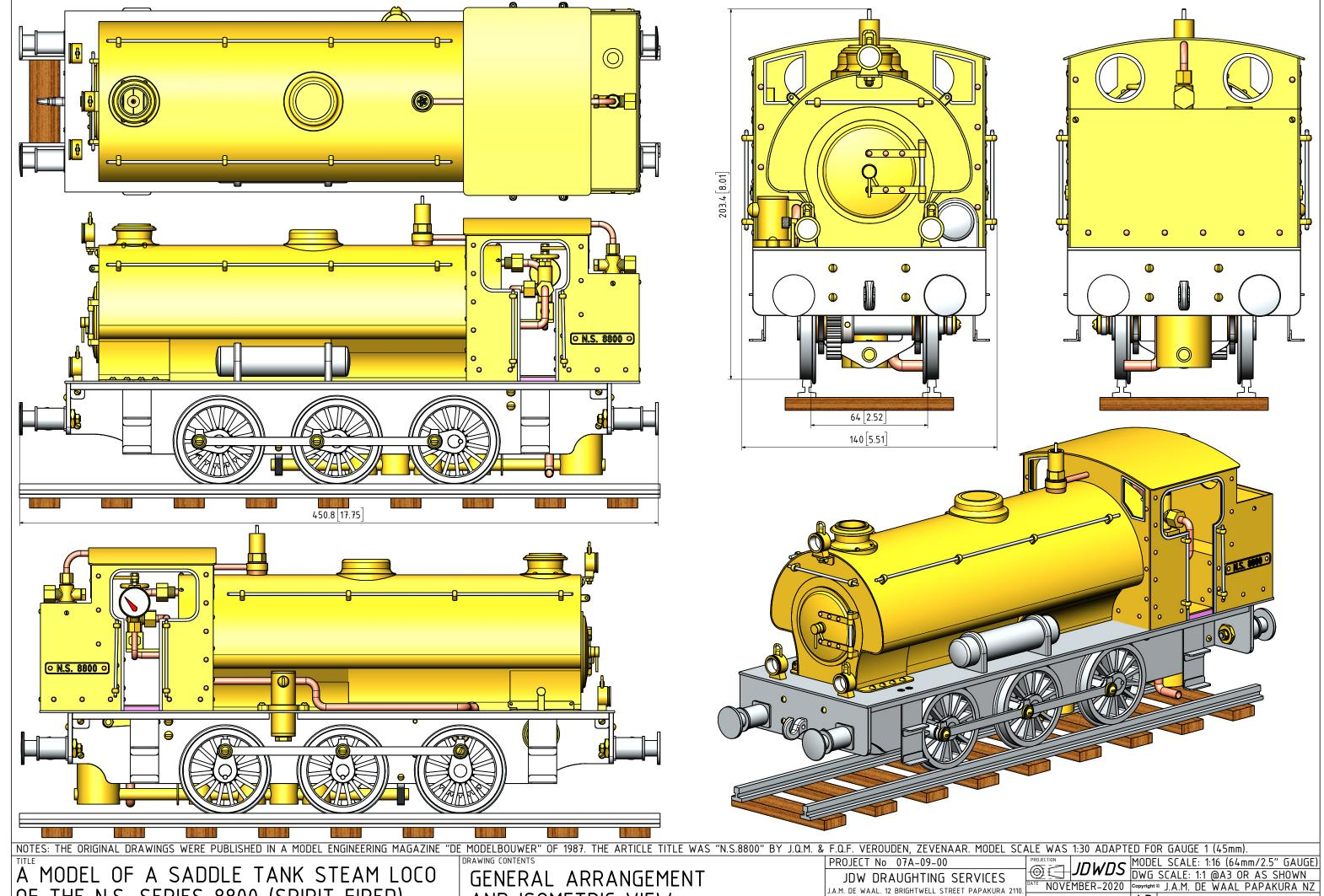
A MODEL OF A SADDLE TANK STEAM LOCO OF THE N.S. SERIES 8800 (SPIRIT FIRED)
